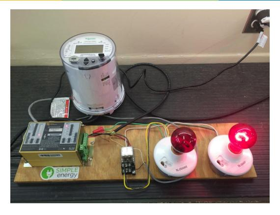
Relay is energized, contact closed, inverter off and status is on
