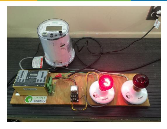
Relay is de-energized in normal state
